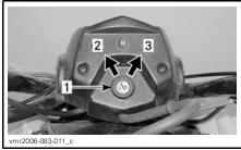
**TYPICAL** — IGNITION SWITCH POSITIONS 1. Ignition switch
